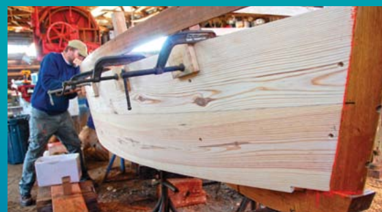
The push boat for the Skipjack Rosie Parks is being restored at Chesapeake Bay Maritime Museum in St. Michaels, MD. Photo by CBMM
