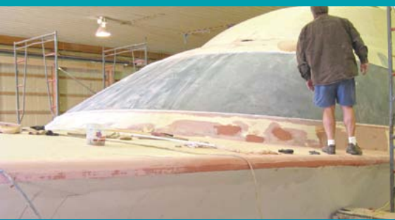
At F&S Boatworks in Bear, DE, a 75-foot cold molded Sportfisherman is taking shape. Photo by Rick Franke
