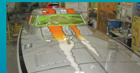
Tug It ’s deck looks as if it’s made of welded and bolted aluminum plates—an illusion created by fades and airbrushing on a smooth deck. Photo by Rick Franke
