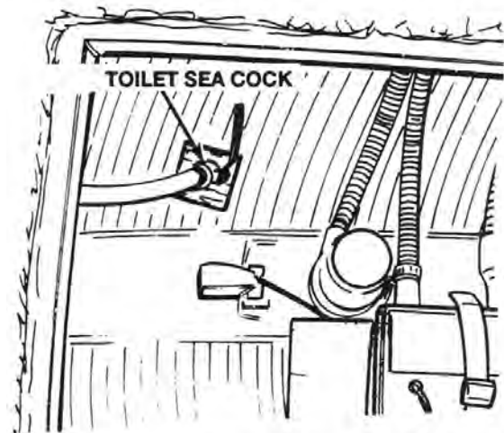
Figure 3-27 - Toilet Sea Cock
